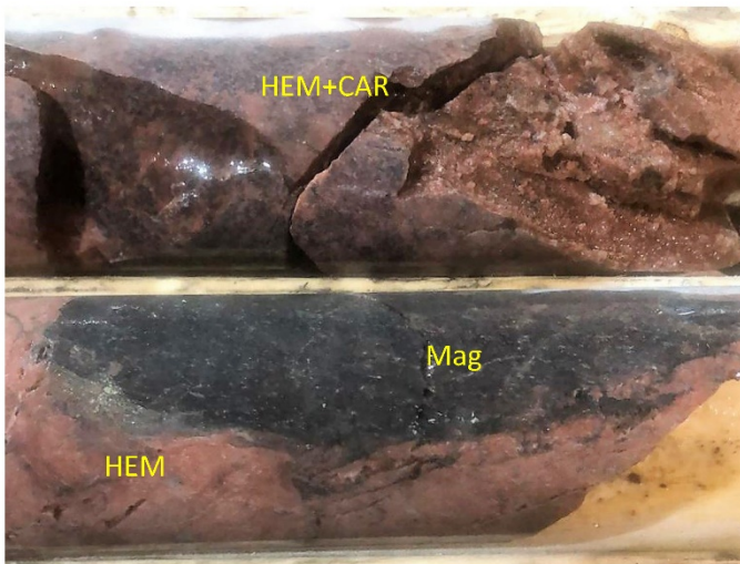
Picture 03: Strong pervasive hematization associated with massive magnetite and fine grained pyrite in hole AP-22-002
