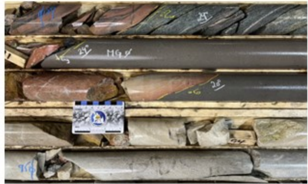
Picture 04: Lamprophyre dyke illustrating the deep root of the regional fault necessary for a magmatic heat source
